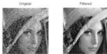
Figure 2.5: Median filtering
